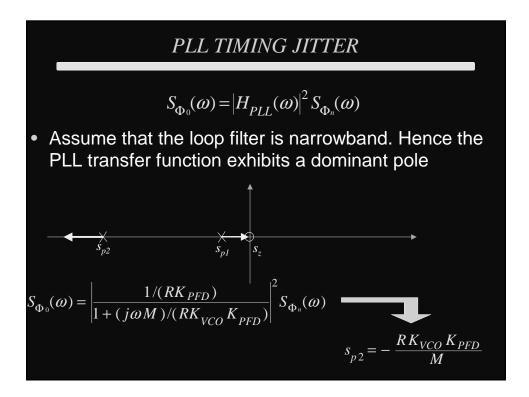
$$\begin{aligned} pLL\ TIMING\ JITTER\ (cont'd) \\ jitter_{\Phi_0}(\tau) &= \sqrt{\left(\frac{K_{VCO}^2}{2K_{PFD}} \frac{\sigma_{Vn,\max}^2}{sp_2^2 t_r}\right) (1 - \exp(-sp_2|\tau|))} \\ Impulsive\ noise \end{aligned}$$
