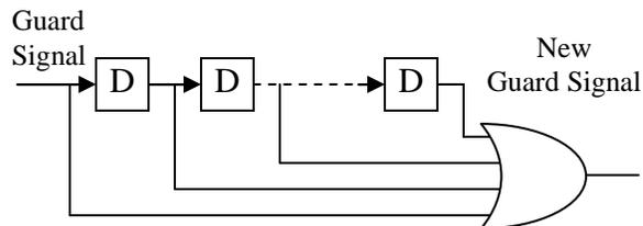
**Figure 8. Limiting the switching frequency of the guarding signal.**
