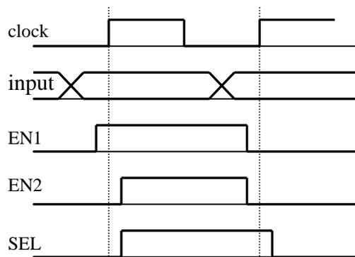
**Figure 5. Timing diagram of the guarded adder circuit.**
