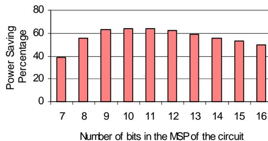
**Figure 9. Power saving for a 32-bit comparator.**
