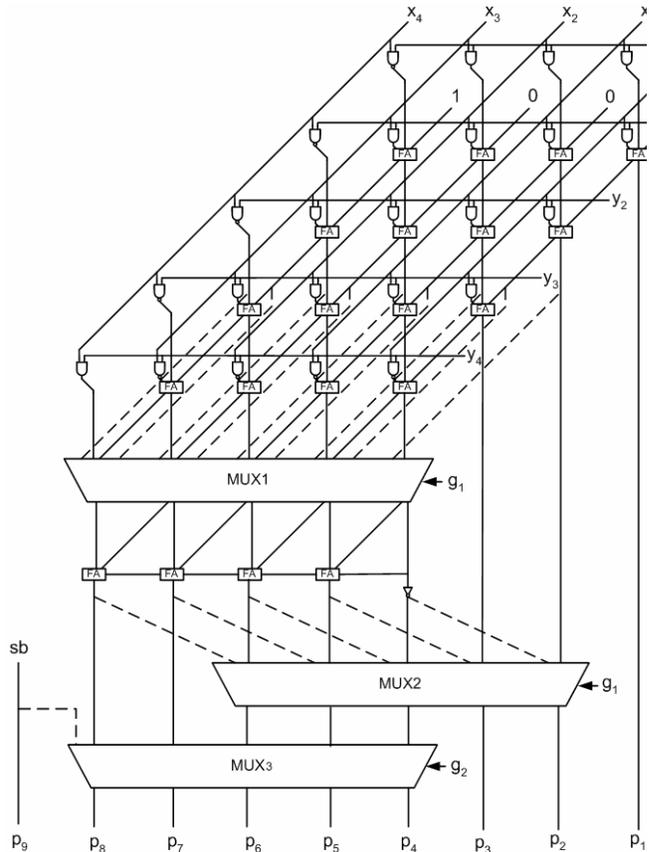
Figure 7. The precomputation-based guarding for a multiplier.
