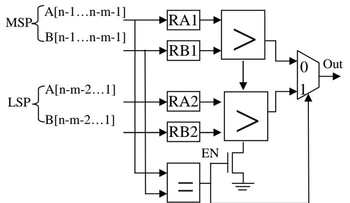
Figure 3. The  $m$ -bit precomputation-based guarding for an  $n$ -bit comparator.
