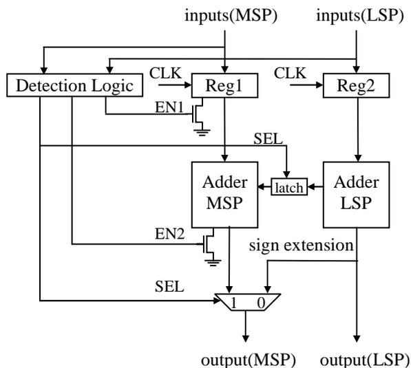
**Figure 4. The precomputation-based guarding for an adder.**
