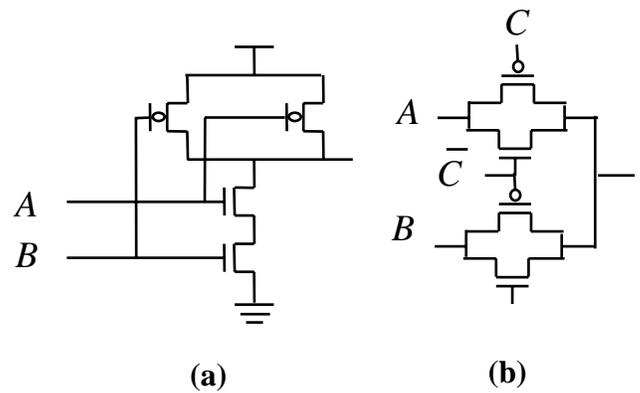
Figure 2. Two circuits that may consume static power after guarding.
