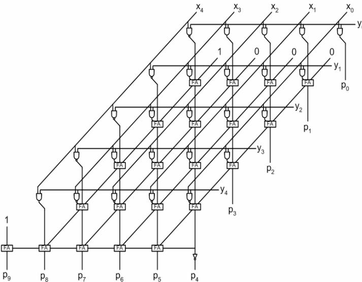
Figure 6. A multiplier using CSA array and one CPA.
