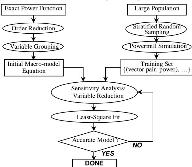
**Figure 1** The workflow of generating a cycle-accurate macro-model
