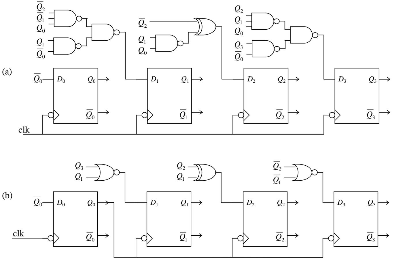
**Fig 4. BCD code up-counter by gating clock (a) asynchronous design, (b) synchronous design**
