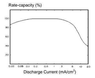
Figure 3 The rate-capacity of the battery
