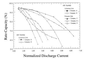
Figure 5 The rate-capacity for commercial NiMH batteries
