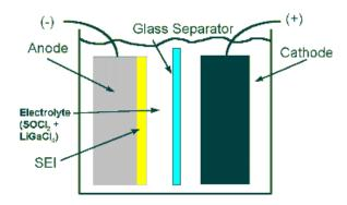
Figure 2 A Lithium battery cell
