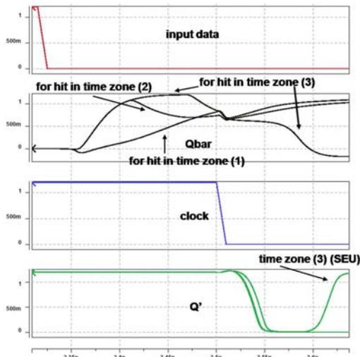
Figure 5. Voltage evolution of  $Q_{bar}$  node in different timing zones
