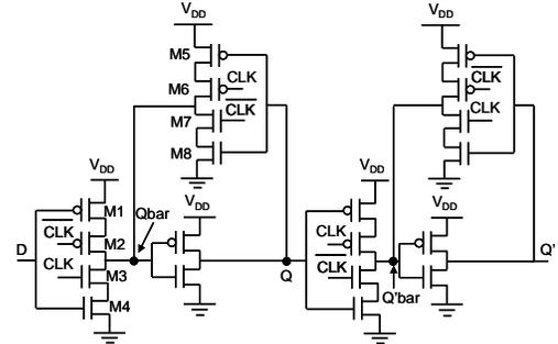
Figure 1. Schematic of a negative-edge triggered C<sup>2</sup>MOS FF.
