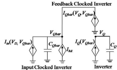
Figure 2. Current based model of a latch
