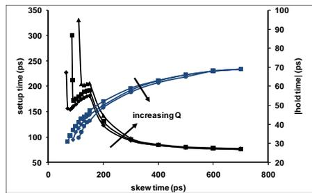
Figure 3. Setup and hold times dependency on  $t_{skew}$  and  $Q$
