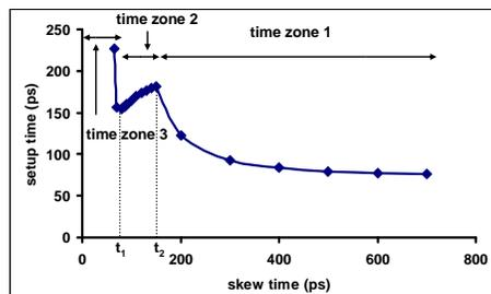
Figure 4. Three different timing zones for particle hit
