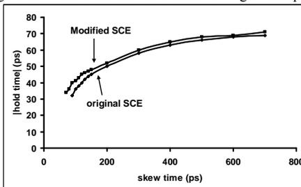
Figure 7. Effect of selective transistor sizing on hold time
