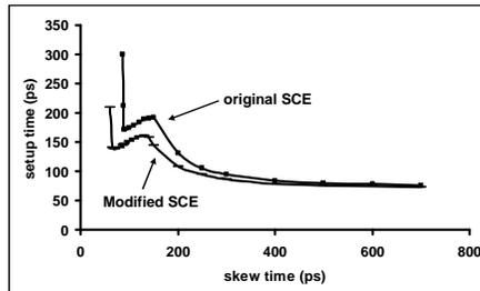
Figure 6. Effect of selective transistor sizing on setup time
