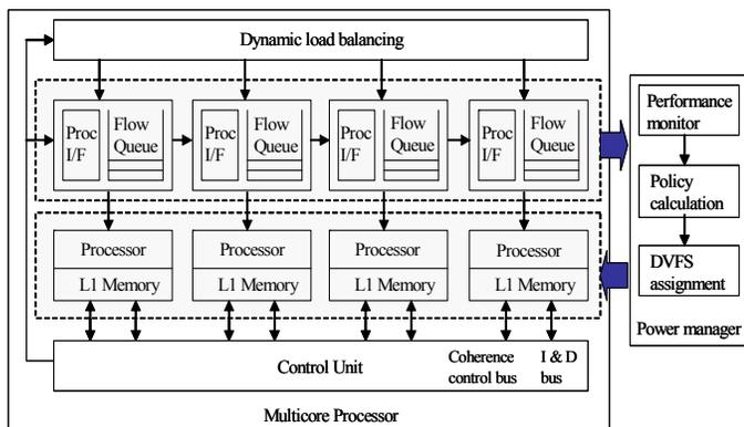
Fig. 1. Example of a power-managed multi-processor system.
