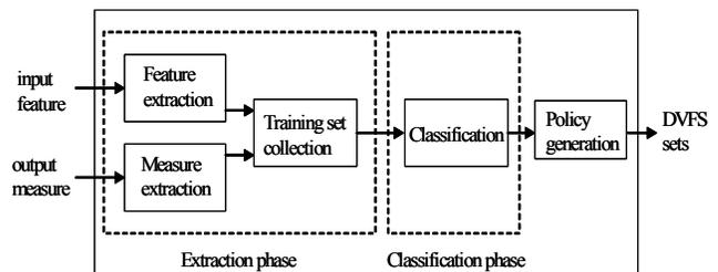
Fig. 3. Structure of the proposed power manager.
