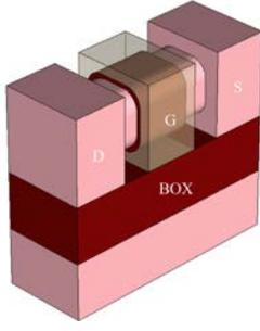
Fig. 1 3D device structure for JL-GAA in TCAD device simulation.
