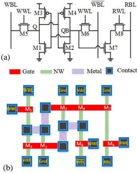
Fig. 5 8T SRAM circuit (a). schematic picture, (b) layout.
